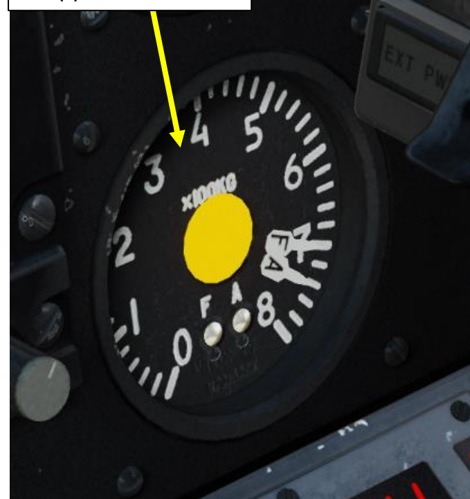
Fuel Indicator (x100 kg) • П (F): Forward Tank Needle • З (A): Aft Tank Needle
