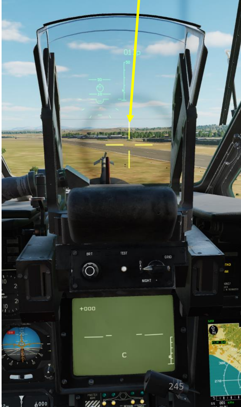
Helmet Mounted Sight Reticle (Gun Armed / Safety Off)
