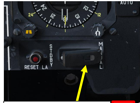
Laser Mode Selector Laser Designator (STDBY) Laser Rangefinder (MANUAL)
