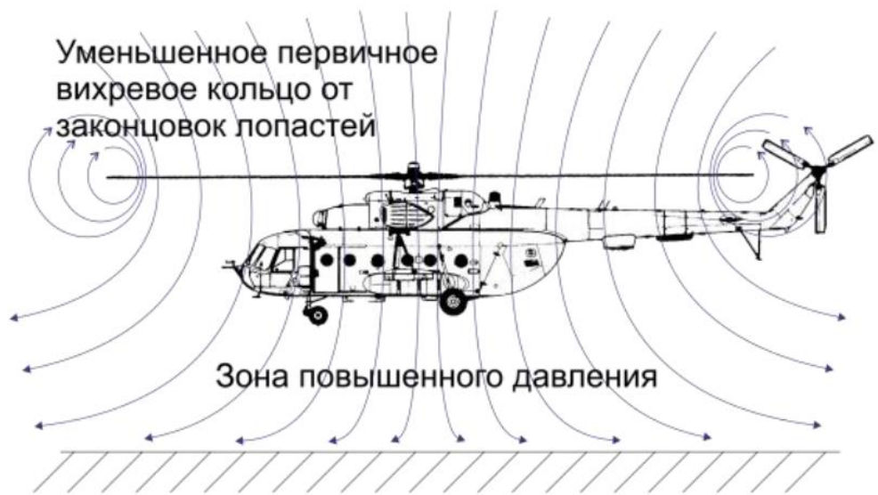
Airflow when In Ground Effect (IGE) (Mi-8)
