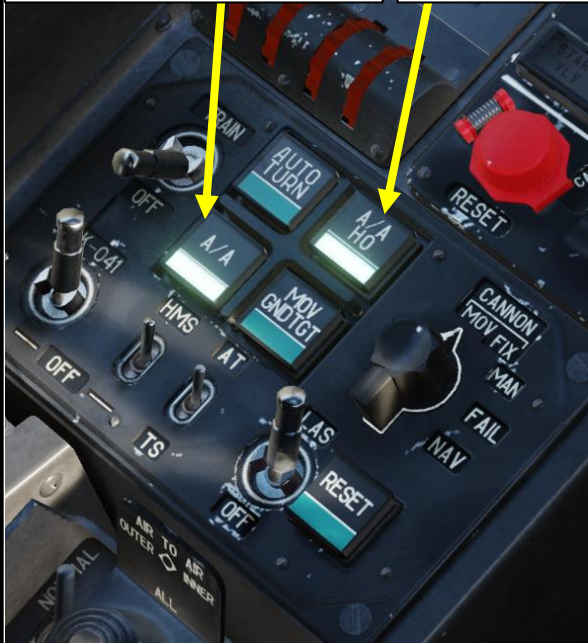
Target Mode Selector Button Air-to-Air
