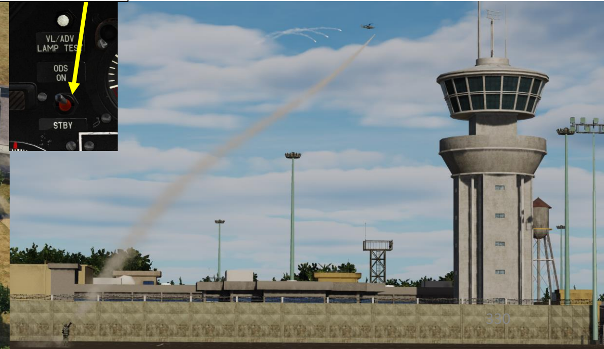
ODS (Onboard Defense System) Mode Selector Switch • UP = ODS ON (Combat Mode) • DOWN = STBY (Standby Mode)
