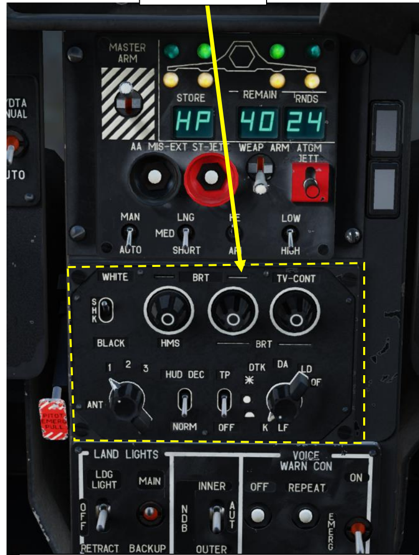
Laser Mode Selector • Laser Designator (STDBY), used to designate targets for weapons such as the Kh-25ML, Kh-29L or laser bombs. Does not affect Vikhr employment. • Laser Rangefinder (MANUAL)
