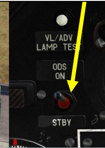
ODS (Onboard Defense System) Mode Selector Switch • UP = ODS ON (Combat Mode) • DOWN = STBY (Standby Mode)
