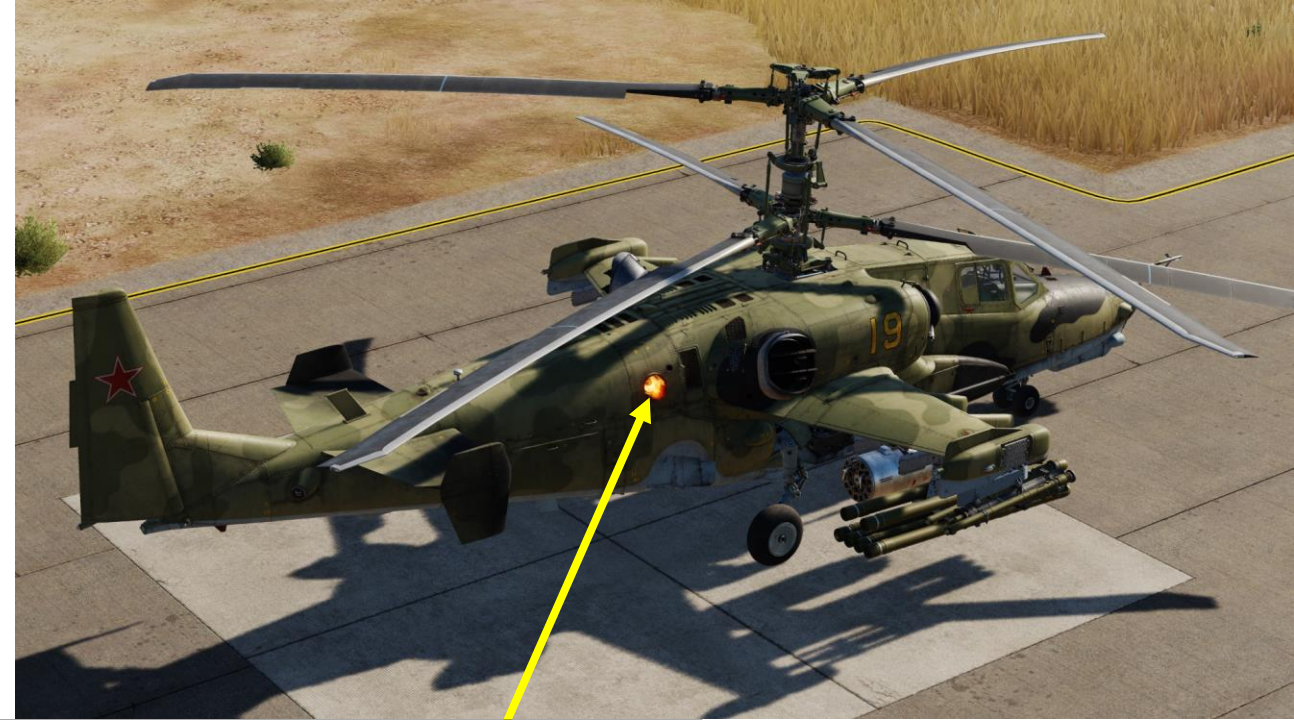
Exhaust Nozzle of Operating APU (Auxiliary Power Unit)
