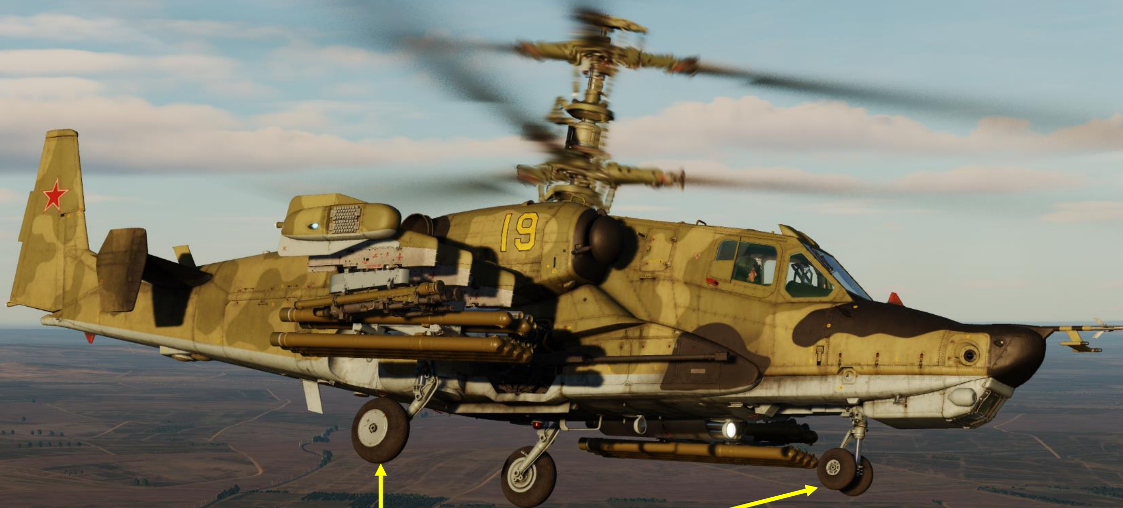
Retractable Landing Gears (Hydraulically actuated)
