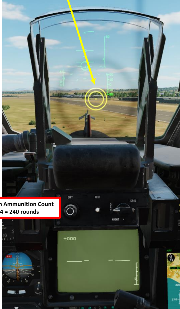
Helmet Mounted Sight Reticle (Gun Not Armed / Safety On)
