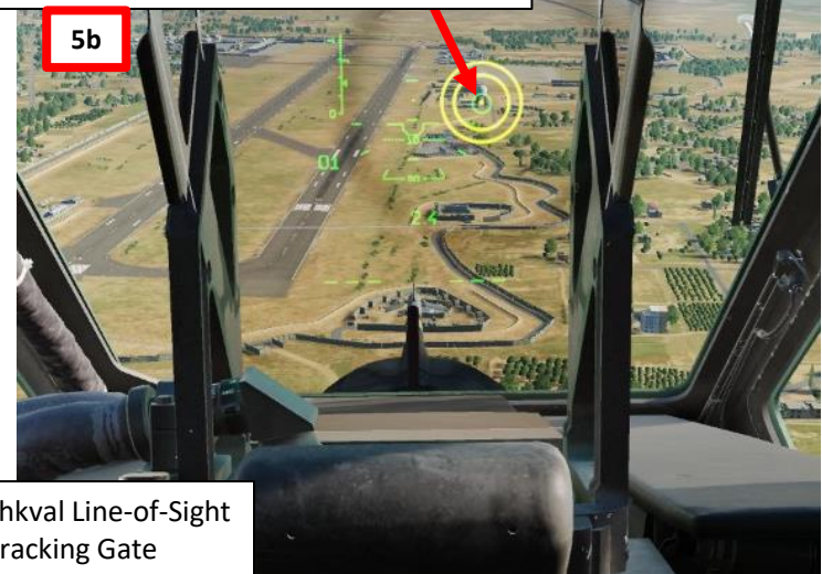
Shkval Line-of-Sight Circle (Green) (Blinks when out of the HUD's field-of-view)
