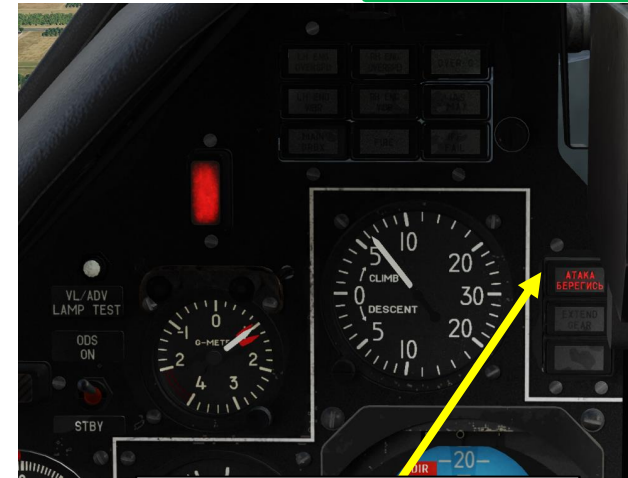
Laser Lock / Missile Warning Light
