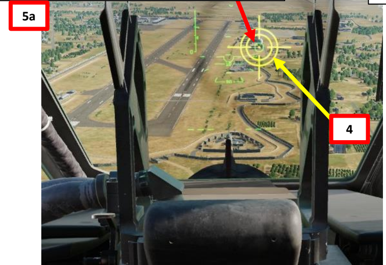
Shkval Line-of-Sight (slaved to HMS Reticle while "Shkval Uncage Button" is pressed)
